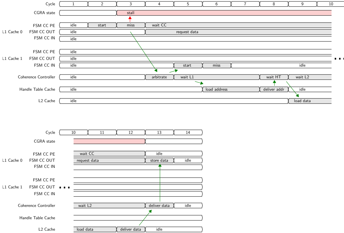
Figure 13.5.: Timing of a L1 cache miss where the desired data can be provided by the L2 cache
