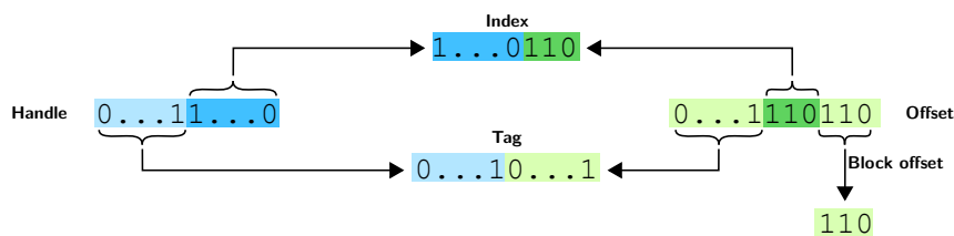
Figure 11.2.: Scheme of index and tag generation in a virtually addressed cache
