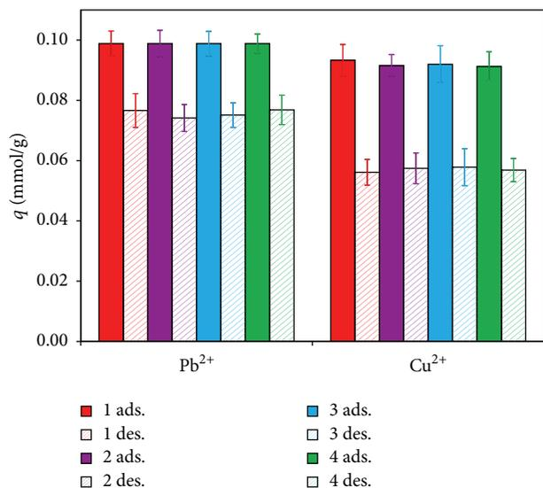
FIGURE 3: Adsorption-desorption cycles of Pb<sup>2+</sup> and Cu<sup>2+</sup> using calcium chloride. Experimental conditions: 0.1 mM initial metal concentration, pH 4.5, and 25°C. Error bars represent standard deviation of triplicate measurements.
