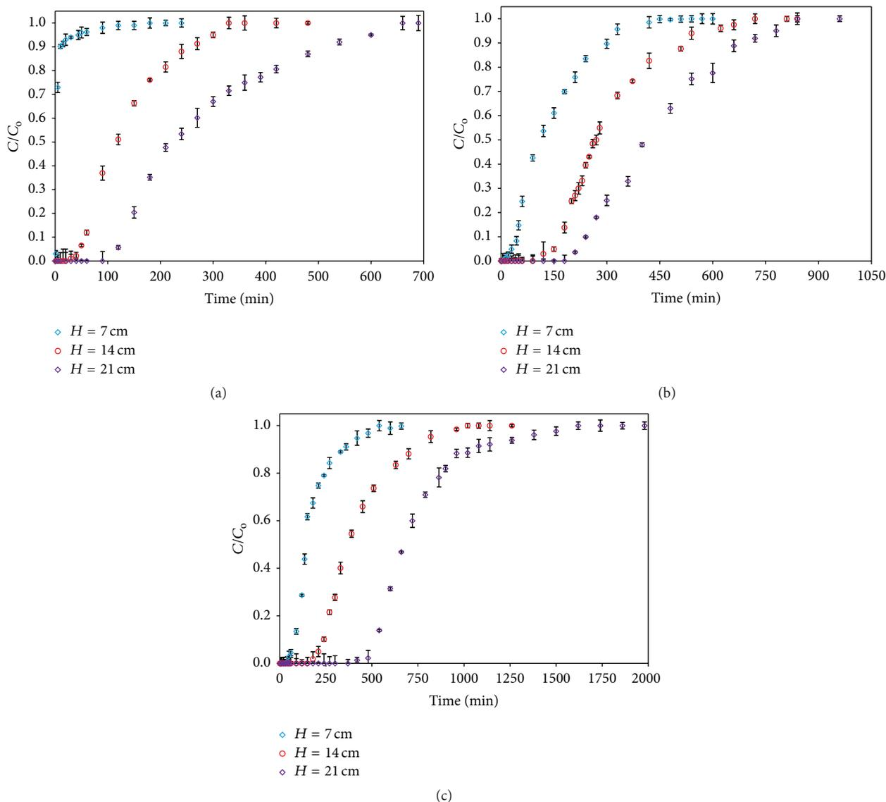
FIGURE 7: Effect of the bed height on the breakthrough curves of (a)  $\text{Cd}^{2+}$ , (b)  $\text{Cu}^{2+}$ , and (c)  $\text{Pb}^{2+}$ . Experimental conditions: 0.1 mM initial metal concentration, pH 4.5, and 25°C.
