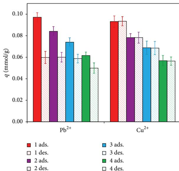
FIGURE 2: Adsorption-desorption cycles of Pb<sup>2+</sup> and Cu<sup>2+</sup> using citric acid. Experimental conditions: 0.1 mM initial metal concentration, pH 4.5, and 25°C. Error bars represent standard deviation of triplicate measurements.
