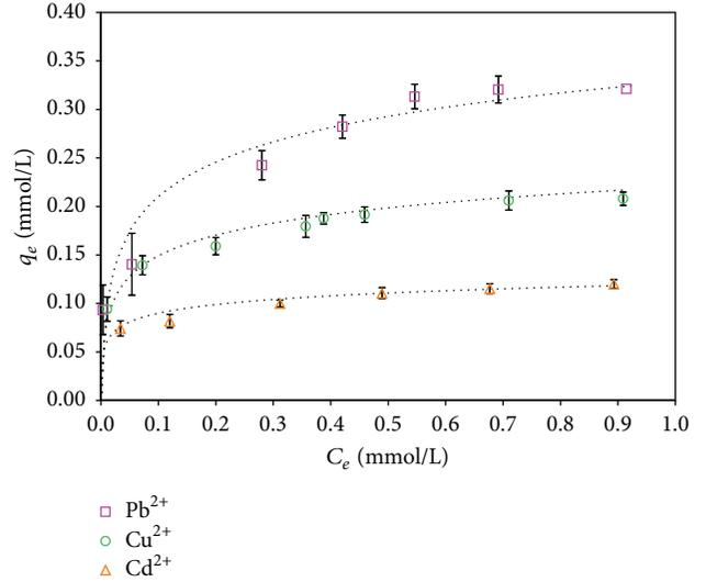
FIGURE 1: Isotherm adsorption of  $\text{Cd}^{2+}$ ,  $\text{Cu}^{2+}$ , and  $\text{Pb}^{2+}$  onto SCG. Experimental conditions: 1 g SCG/L, pH 4.5, and  $25^\circ\text{C}$ . Solid lines represent the ion-exchange multicomponent model. Error bars represent standard deviation of triplicate measurements.
