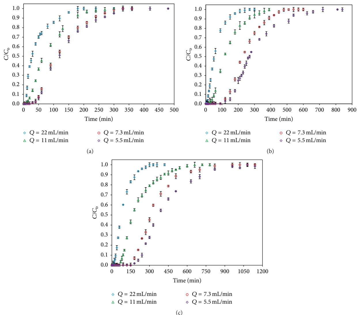
FIGURE 6: Effect of the flow rate on the breakthrough curves of (a)  $\text{Cd}^{2+}$ , (b)  $\text{Cu}^{2+}$ , and (c)  $\text{Pb}^{2+}$ . Experimental conditions: 0.1 mM initial metal concentration, pH 4.5, and 25°C.
