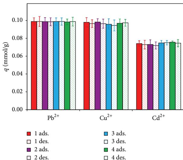
FIGURE 4: Adsorption-desorption cycles of Pb<sup>2+</sup>, Cu<sup>2+</sup>, and Cd<sup>2+</sup> using nitric acid. Experimental conditions: 0.1 mM initial metal concentration, pH 4.5, and 25°C. Error bars represent standard deviation of triplicate measurements.
