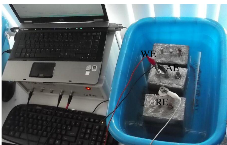
Figure 2. Electrochemical cell for to evaluation of specimens in solution at 3.5% NaCl.
