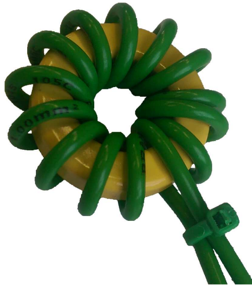
Figure 3.25: A small, low EPC, inductor
