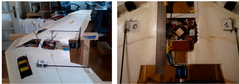
Figure 1. Photos of the electric powered Styrofoam delta shaped fixed wing Unmanned Aerial Vehicle (UAV) used in this study.
