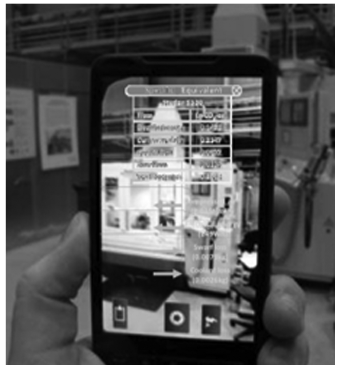
Fig. 8. Use of augmented reality to determine environmental impacts of a manufacturing process [60].
