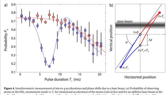
atoms in the  $0\hbar k_L$  momentum mode vs  $T_1$  for minimized acceleration of the atoms (red circles) and for an addition laser beam in the path of the upper wave packets (blue squares). Error bars indicate one standard deviation of the data points. (b) Illustration of the position of the wave packets and the additional laser beam during the pulse sequence. Angles and axes are not to scale in the illustration.
