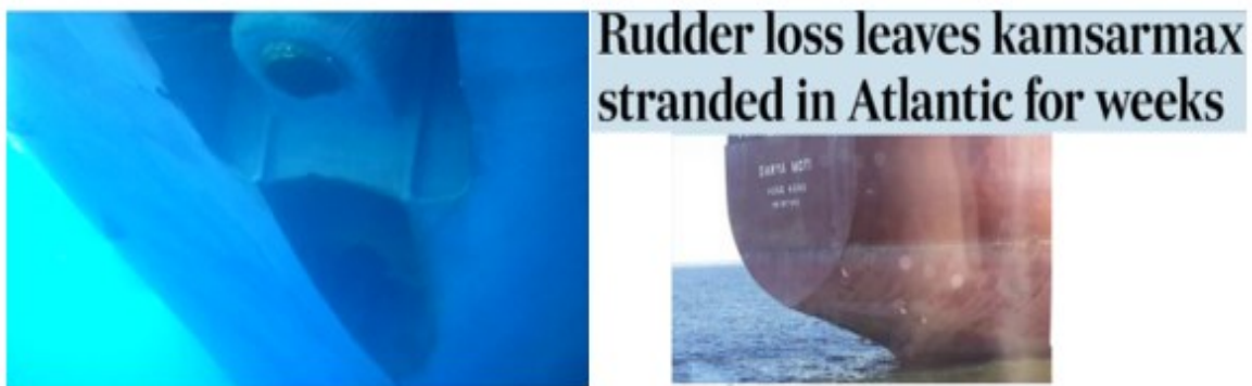
Figure 1 - Rudder loss of a Kamsarmax vessel due to rudder horn failure (TradeWinds, 2014)
