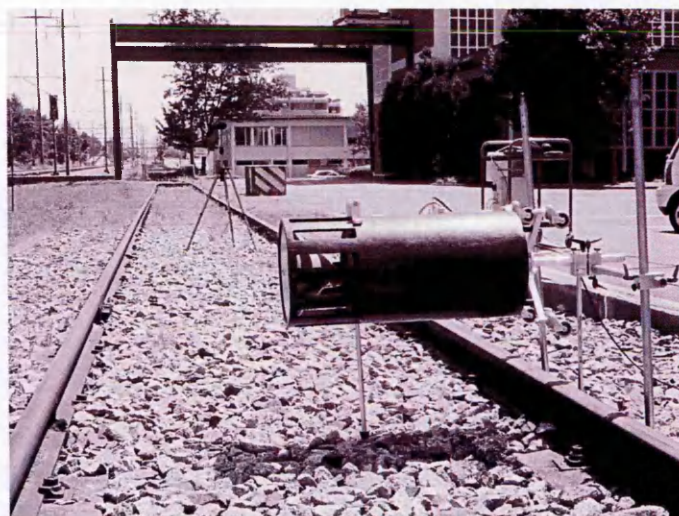
Figure 4.17 Excess attenuation measurement over railway ballast [75].
