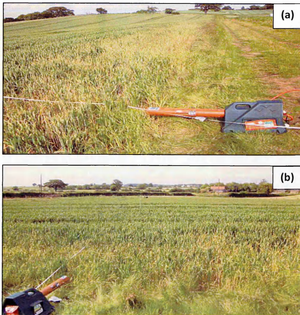
Figure 10.18 Photographs of measurements a using a Propane cannon over winter 0.45 m – 0.55 m high winter wheat crops.
