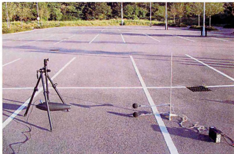
Figure 3.19 Level difference measurement over a hard asphalt ground car park.
