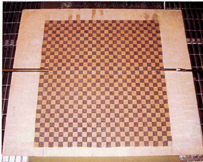
Figure 7.12 Laboratory configurations used to investigate sound propagation over 3D impedance patches. In these photographs the finite impedance is provided by felt.
