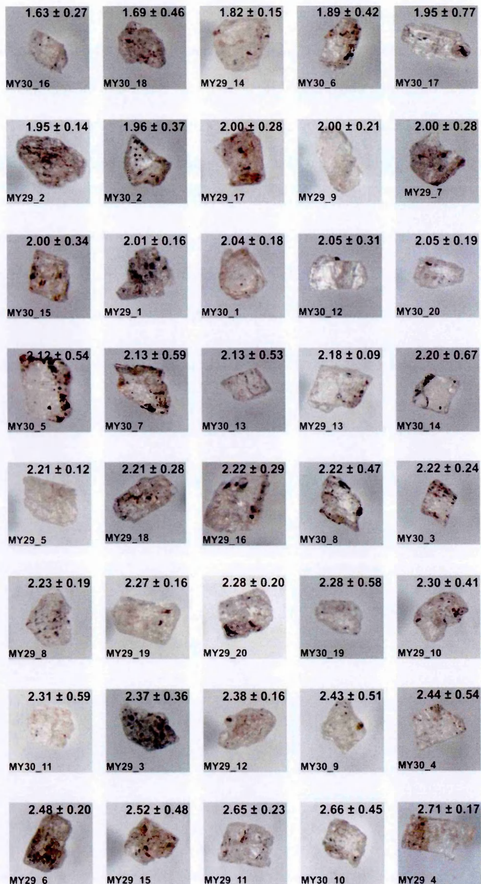
Figure 3.26. Photograph of each Sheridan Reservoir dome feldspar crystal analysed by Ar-Ar single-grain fusion. Analysis number given in the bottom left corner and Ar-Ar apparent age ( \text{Ma} \pm 2\sigma ) is given in the top right corner. Crystal size varies 500 \mu\text{m} to 1 mm in size.
