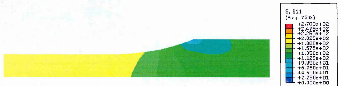
Figure 4.22 Contour plots of predicted stresses in the tensile direction of the initial design (Elastic-plastic analysis result)
