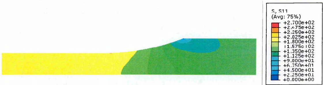
Figure 4.20 Contour plots of predicted stresses in the tensile direction of the new proposed design (Elastic analysis result)
