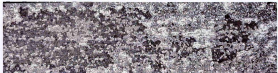
Figure 4.2 Painted specimen surface at 600 °C for 5 months
