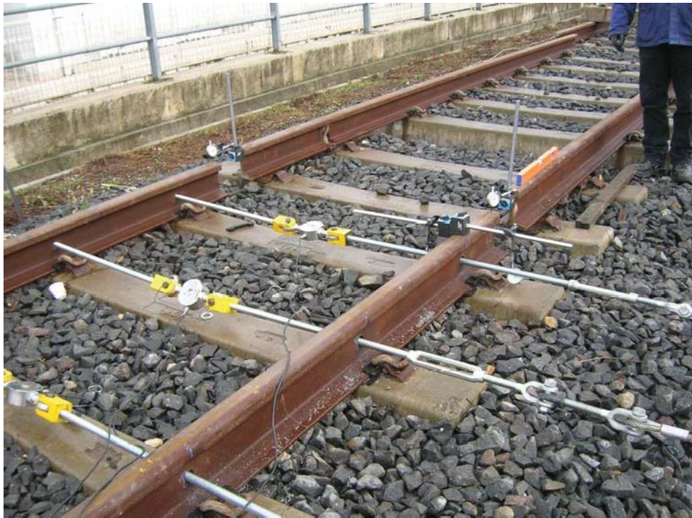
Figure 5. Test on BBB scenario (with ballast shoulder and ballast crib). FIGURE #5 219x164mm (300 x 300 DPI)
