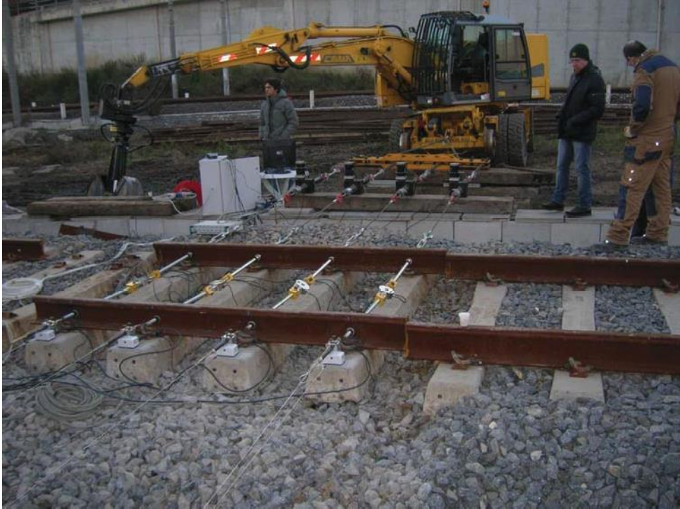
Figure 8. Test on BCU scenario (without ballast crib, C, and at sleepers ends, U). FIGURE #8 219x164mm (300 x 300 DPI)
