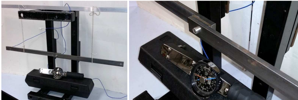
Figure 2: Test structure with torque wrench and joint detail.
