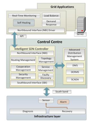
Fig. 1. Digital grid self-healing using intelligent SDN technology.
