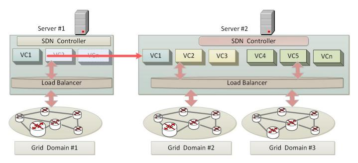
Fig. 2. Load balance and resource distribution between various grid domains.
