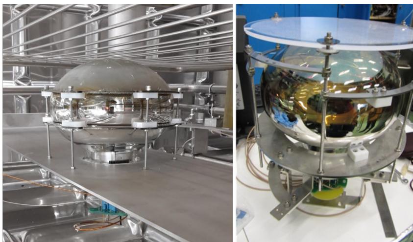
Figure 15. Left: picture of one PMT coated with TPB. Right: a PMT unit with the coated plate mounted in front of the photo-cathode and ready for its installation.
