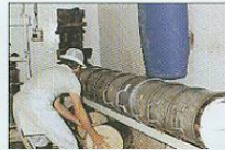
4 Cheddar is pressed in two stages, here in the horizontal press, for 12-16 hours each time.
