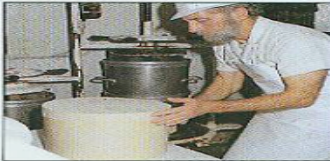
9 Before the second, very hard pressing, the cheese is wrapped in cloth — first, the top and bottom.
