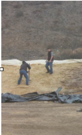
Figure 9. Digging holes to get samples at each depth.
