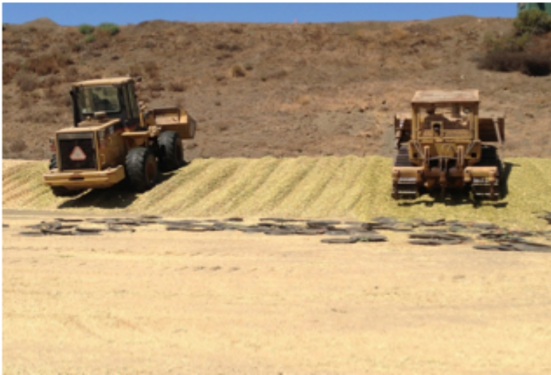
Figure 1. Loader and crawler packing the pit.
