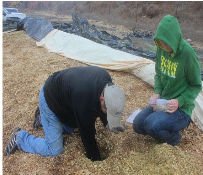
Figure 10. Obtaining samples from 0 to 6, 6 to 12, and 12 to 18 inches from the surface.
