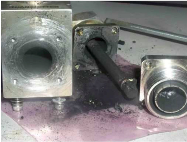
FIG. 17. (Color) Photo of a damaged high-power directional coupler installed on the PEP-II beam line to instrument beam-driven kicker power. While designed to operate at 5 KW power levels, the kicker loads, cables, and feedthroughs were problematic in operation. Three different styles of high-power rf connectors were commissioned in the PEP-II runs, each had high-power difficulties. The beam induced power was spread in a very broad band extending to 20 GHz. Seen in the figure is a damaged and destroyed 9/16 DIN connector and directional coupler port.
