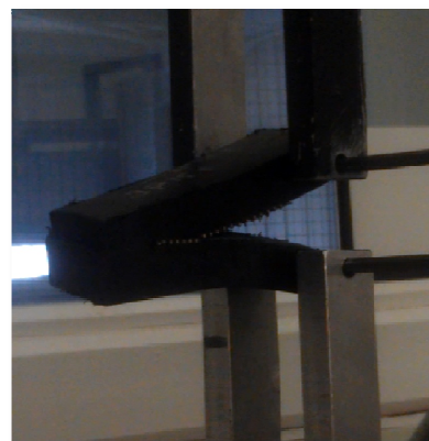
Figure 12: (Left) Instron tensile testing device (Right) Weld being pulled apart during destructive testing
