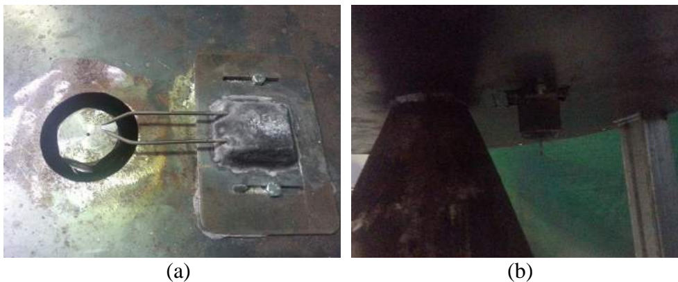
Figure 11. Ignition system: (a) ignition lead top view (inside the burner); (b) bottom view (outside the burner)
