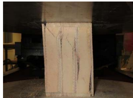
Figure 14. Failure in transverse compression of hybrid FRP composite beam
