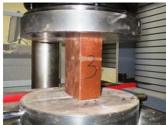
Figure 5. Longitudinal compression test
