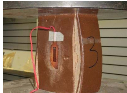
Figure 12. Failure in longitudinal compression of hybrid FRP composite beam
