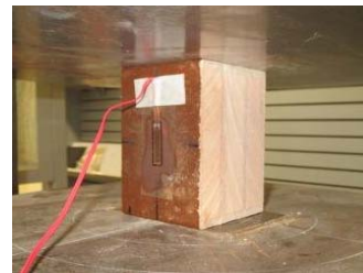
Figure 6. Transverse compression test
