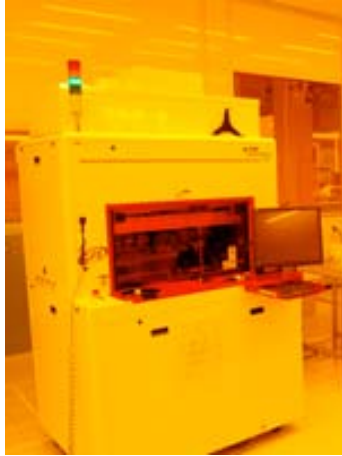
Figure 1.15. Imprio 55, Molecular Imprints, S&F UV-NIL equipment.
