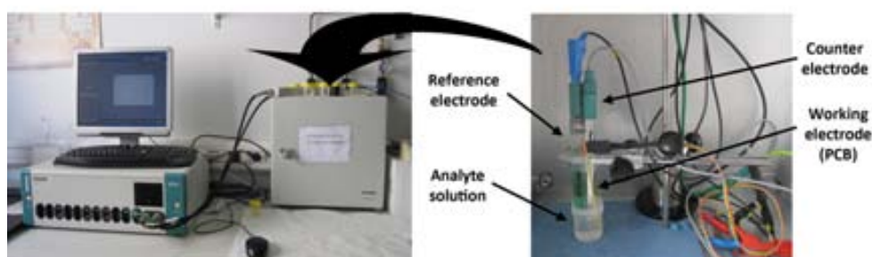
Figure 5.19. Shows complete set-up to perform electrochemical measurements in liquid.
