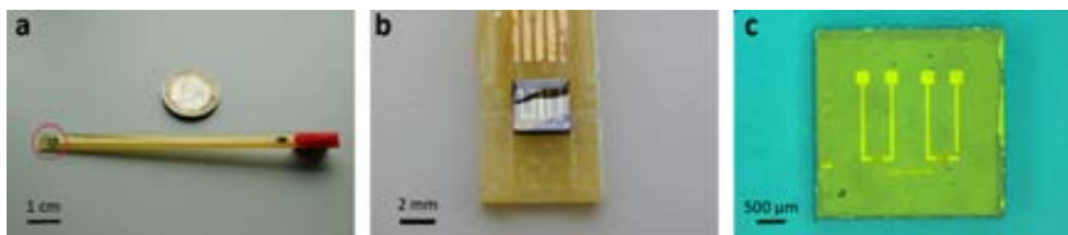
Figure 5.5. Images of the PCB strip packaging. a) Complete PCB. b) Inset of the PCB strip of the area where the chip is placed. Details of the wire bonding can be appreciated. c) Image of 3 \times 3 \text{ mm}^2 single chip with two IDEs, similar to the one placed on the PCB.
