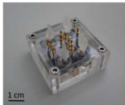
Figure 5.10. Holder type packaging is composed of a methacrylate frame with cavity for a 2 \times 2 \text{ cm}^2 chip and orifices for 4 screws, 10 metallic pins and 4 connector tubes.
