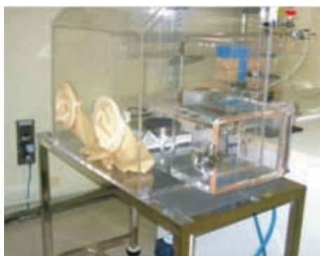
Figure 1.21. Globe box used to deposit silanes under vacuum atmosphere.
