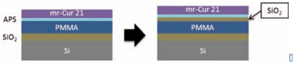
Figure 4.14. Ultrathin layer of \text{SiO}_2 (10 nm) was deposited between the APS and the PMMA to improve the adhesion between both materials.
