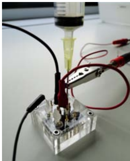
Figure 5.25. Complete set-up of the holder for the IDEs characterization.
