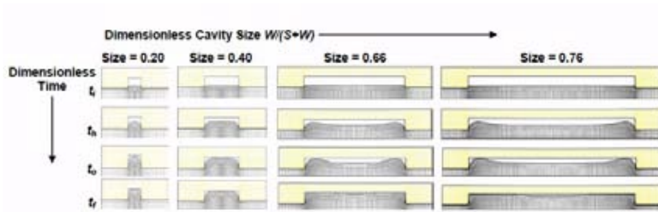
Figure 1.8. Deformation profiles for (a) increasing cavity width holding indenter width and film thickness constant [43].
