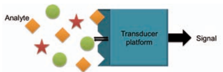
Figure 6.4. Operating principle of a electrochemical sensor
