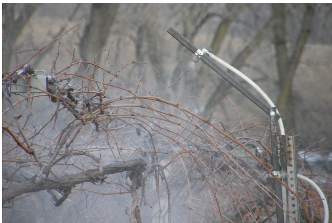
Figure 7. Flat fan spray nozzle attached to the adjustable arms of the sprayer. The small droplets easily penetrate into the cordon area and cover all buds.
