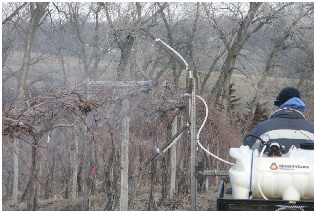
Figure 6. ATV Sprayer modified to spray Amigo Oil and NAA on unpruned vines.
