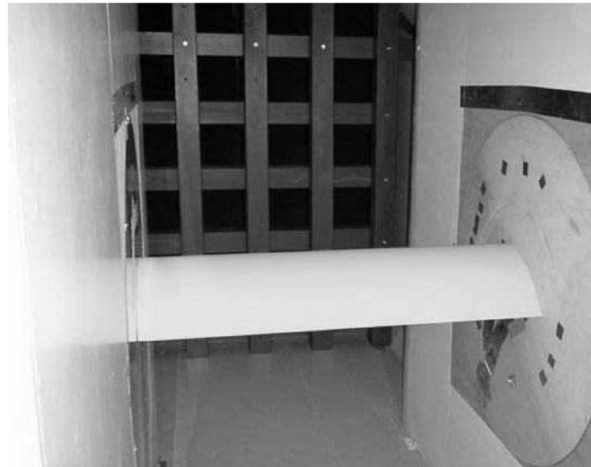
Figure 31 - Square grid set-up - Devinant et al (2002)
