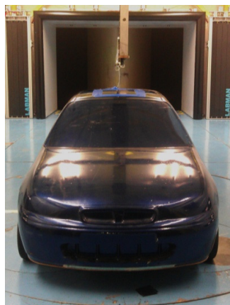
Figure 274 - Rover 200 40% model in Durham University's 2m wind tunnel
