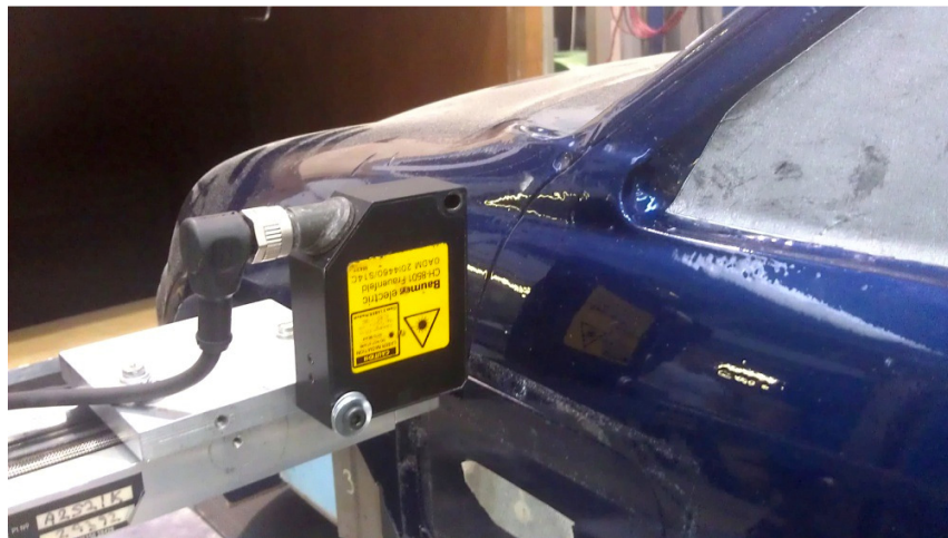
Figure 272 - Laser distance measuring device, Baumer, 30–130mm range, on 3-axis traverse
