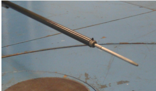
Figure 214 - Laser sintered probe with carbon fibre arm
