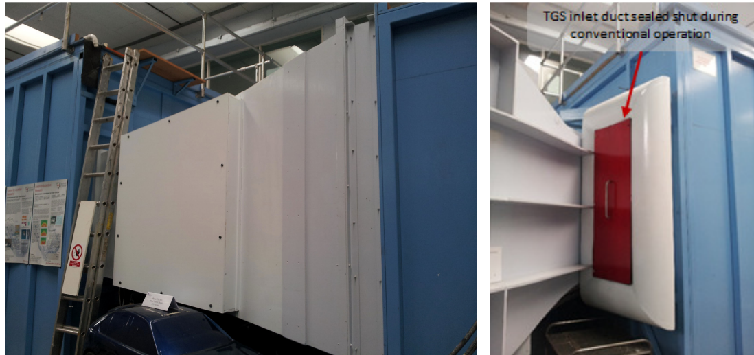
Figure 193 - Additional inlet and exhaust ducting to feed the TGS front and rear shutter units
