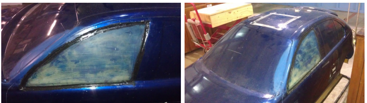
Figure 273 - Rover 200 model with sideglass tappings
