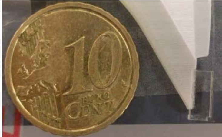
Figure 4-1: Customised probe used in \mu DMA testing
