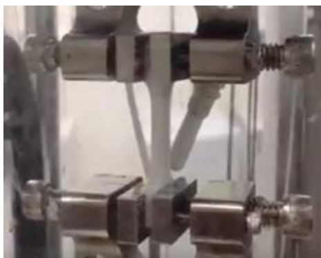
Figure 4-4: Testing of a Quadrathane with a radiopacifier (barium sulfate)
