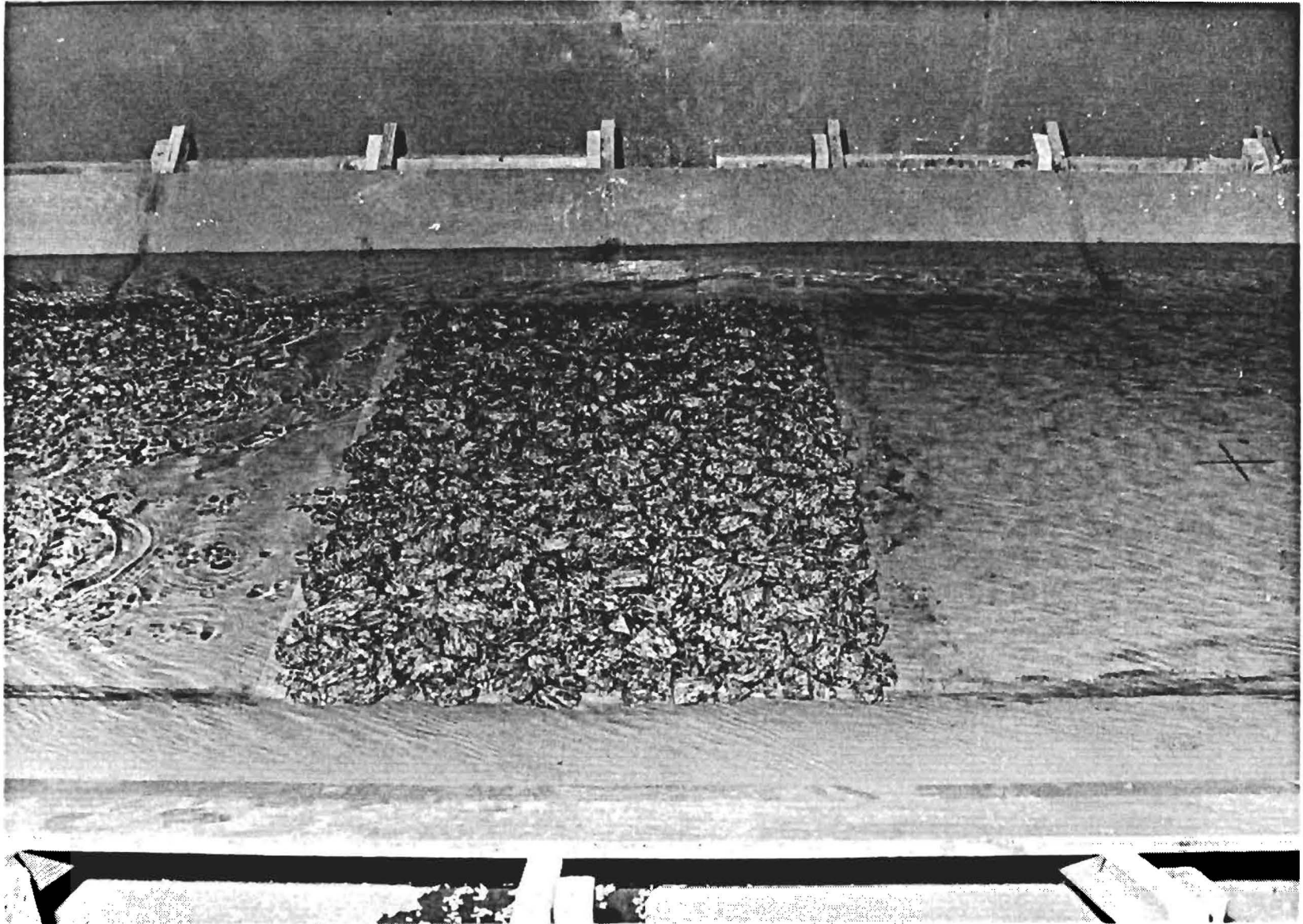
Fig. 14-Close-Up View of Flow (Right to Left) Over 10-ft Weir; Q=25,000 cfs; Tailwater Elevation=68 ft
