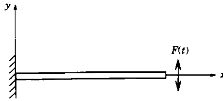
Figure 1. The co-ordinate system of a cantilever beam excited by a harmonic force.
