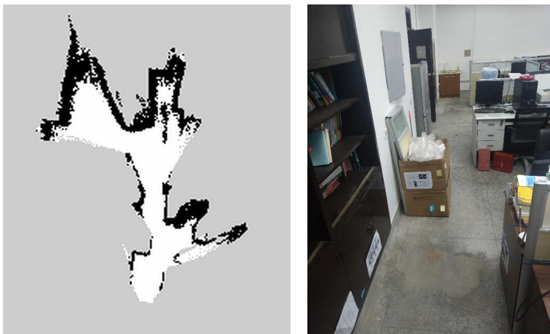
Fig.4.19 2D Map Generated by VSLAM Algorithm
