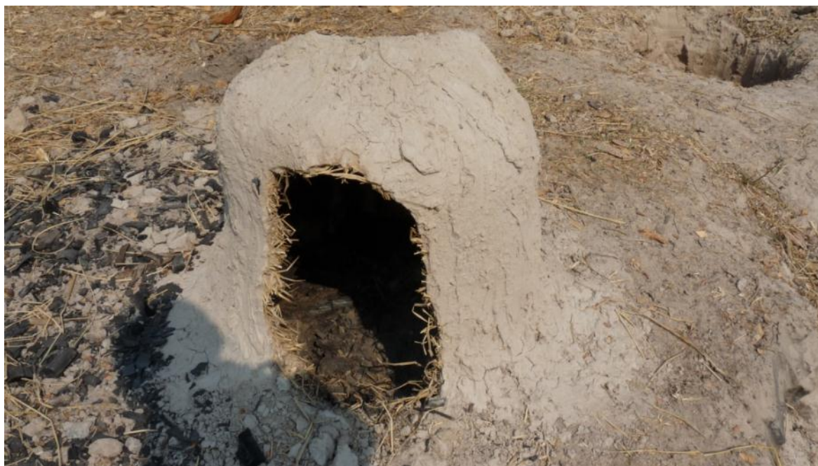
Picture 7. An oven for charcoal production in Vangkaben village, Savannakhet.
