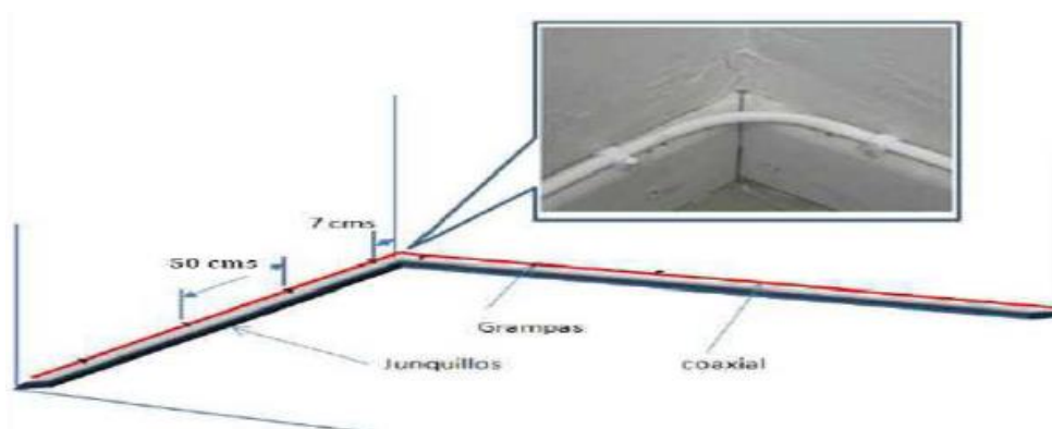
Figura 86. Tendido interior de cable coaxial
