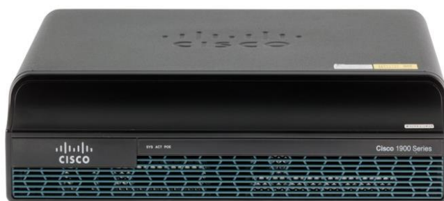
FIGURA 3. 6: Cisco 1941 Integrated Services Router.
