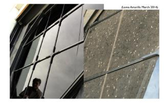
**Figure 4.7:** A picture of the UV filter of Loma Amarilla in March 2014 before (right) and after (left) cleaning. Figure from [106].
