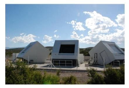
**Figure 3.7:** Photograph of HEAT telescopes tilted upward [77]. The first and the third telescopes with closed shutters and the shutter of the second telescoped is opened for cleaning.
