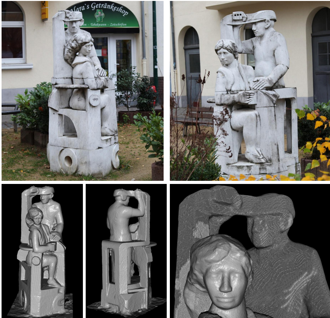
Figure 4.12: Two input images of the Kopernikus data set, the complete reconstructed model from two perspectives and a close-up of the wireframe showing the adaptively triangulated mesh.
