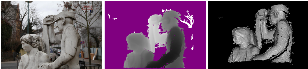
Figure 4.1: Left: An input image to multi-view stereo reconstruction. Middle: The reconstructed depth map visualized in gray values (white: far, black: near). Right: The triangulated depth map rendered from a slightly different view point.
