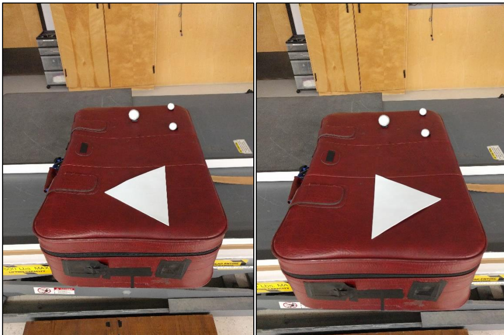
Figure 3. 2 Horizontally placed suitcase with the two visual cue types. 3.2a (left) shows CUE LEFT where the arrow head points towards the left side. 3.2b (right) shows CUE RIGHT with the arrow head pointing towards the right side. Three reflective markers were also placed on the suitcase in order to track the suitcase's movement in motion capture.
