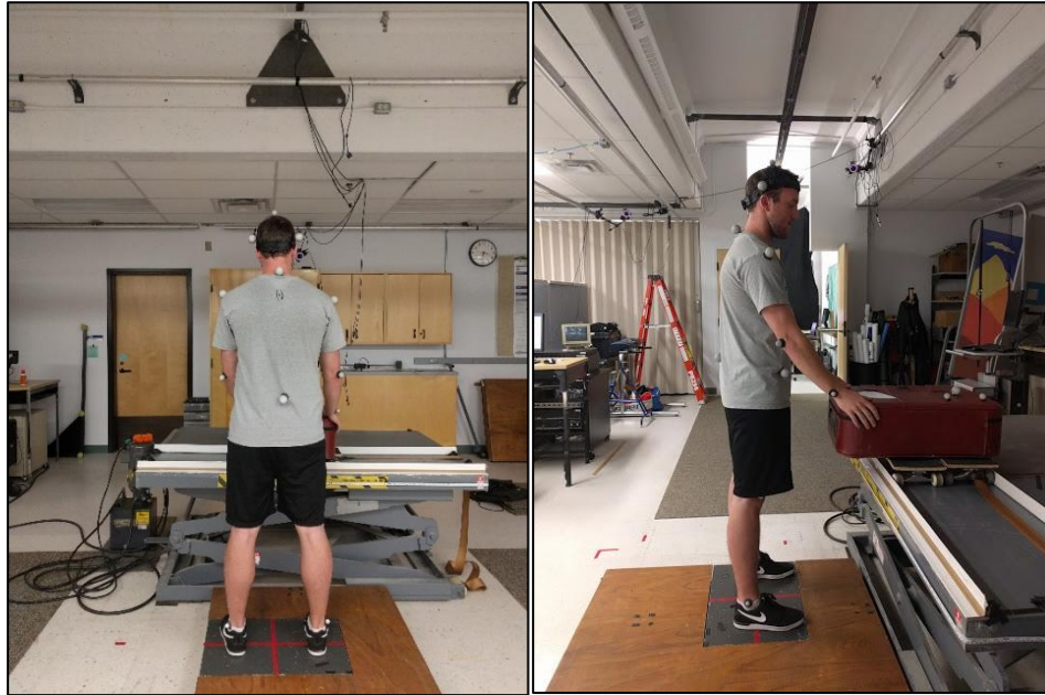
Figure 3. 1 The experiment 3 setup. 3.1a (left) shows the posterior-anterior view of a participant standing on a force platform. 3.1b (right) indicates the lateral view of the participant with the suitcase placed horizontally on a sliding rail ready for pulling motion. Participants' were marked up with reflective markers for motion capture.
