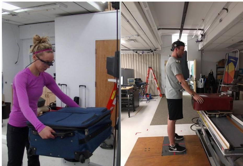
Figure 1. 3 Recreating a suitcase handling work task in the laboratory with different bio-instruments in order to analyze the various factors associated in occupational handling tasks. On the left, the subject is wearing a pair of vision tracking goggles that keeps track of her visual attention during a suitcase handling task. On the right, the participant is equipped with reflective markers on his body in order to track his biomechanical motion using motion capture. He is also standing on a force platform that keeps track of his kinetic profile during the handling task.
