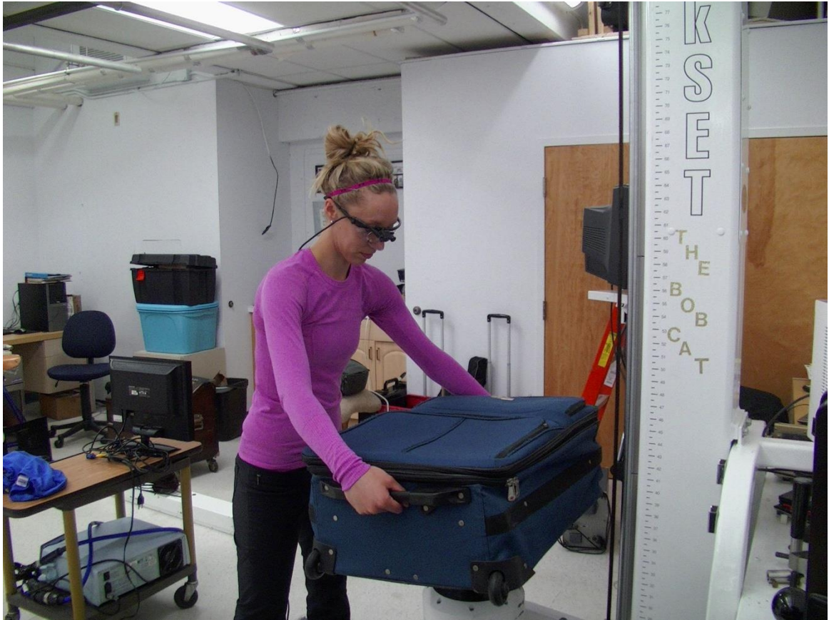
Figure 2. 1 Suitcase orientation during the handling task. The suitcase is placed on a LIDO dynamometer while the subject is also equipped with vision tracking goggles.
