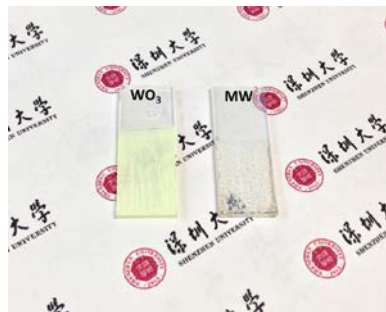
Figure S11 The \text{WO}_3 and MW fabricated onto electrode on a FTO by electrophoresis method.
