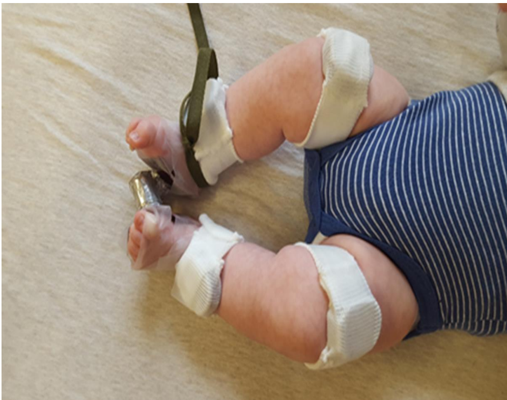
Figure 2. An exemplar infant with bilateral foot markers and 3-D wireless sensors attached to the anterior-distal aspect of the infant's thighs and shanks.
