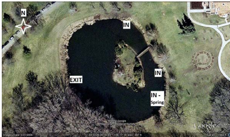
Figure 1. Aerial photo of Dew Drop Pond, St. Paul, MN. Photo was taken in March 2006. IN = drain inlet; IN – spring = freshwater spring inlet; EXIT – exit stormwater drain.
