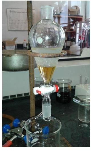
Extraction Set-Up Using brine and CH<sub>2</sub>Cl<sub>2</sub>
