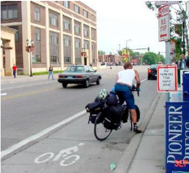
(c) Bike Lane with Gutter and Curb 29
