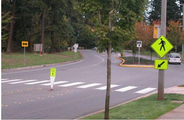
Markings at Mid-block Pedestrian Crossings
