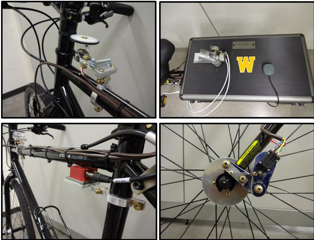
Figure 3-2: Close up view of each of the sensors used on the IPB: Steering Angle (top left), Rider Position and GPS Antenna (top right), IMU (bottom left), Wheel RPM (bottom right).
