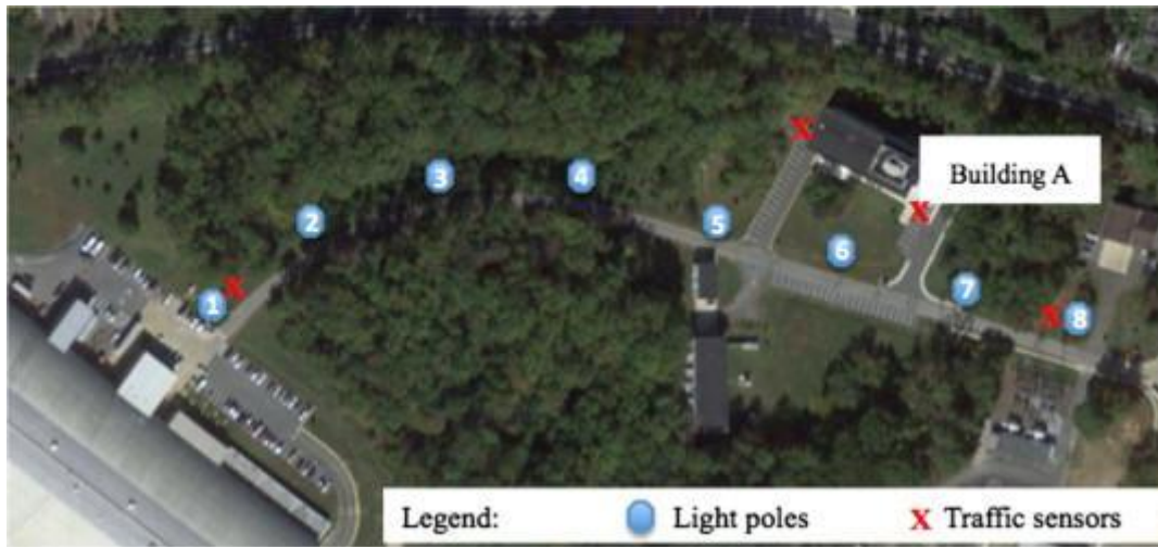
Figure 5-3. Light poles and traffic sensor arrangement (Pipattanasomporn et al. 2014)
