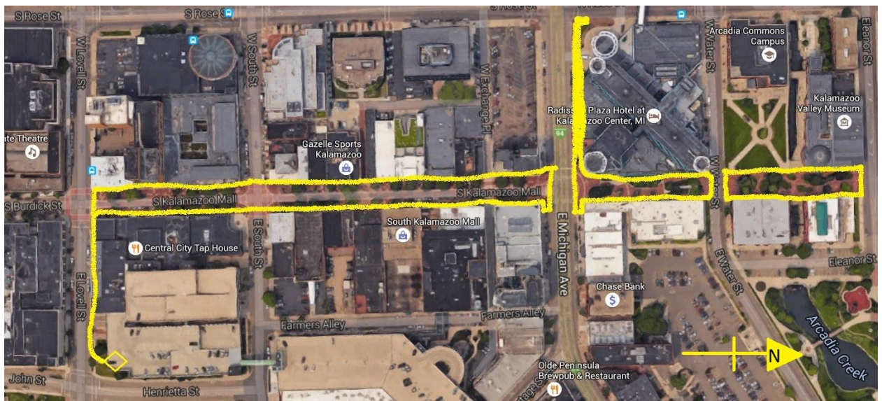
Figure 5-30. Kalamazoo mall snowmelt system coverage area
