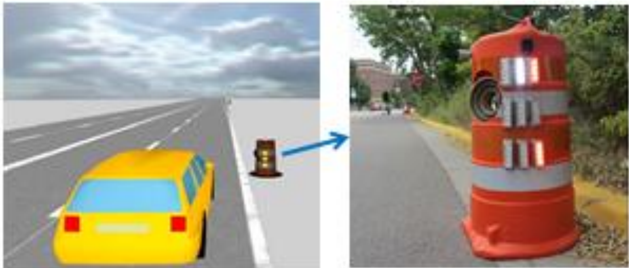
Figure 2-32. Intelligent drum line system (Hourdos 2012)
