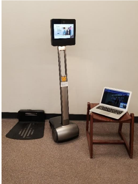
Figure 1. The Beam telepresence robot with charging station and software connection via laptop.
