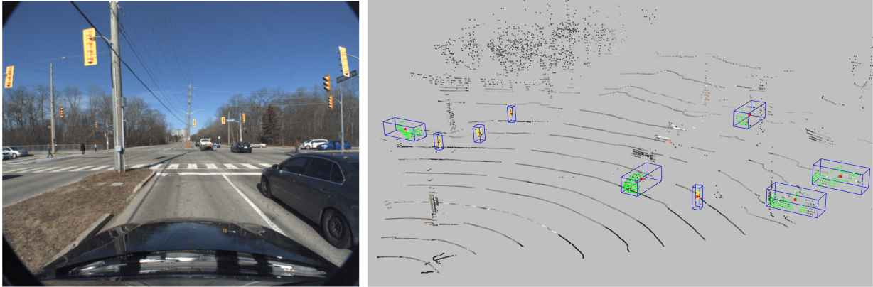
Figure 4.9: Qualitative results of the annotation scheme on data collected by the Autonomoose autonomous vehicle. Instance level segmentation results for the three classes are depicted in green for cars, yellow for pedestrians and cyan for cyclists. Centroid estimation is depicted in red and the final 3D bounding box is depicted in blue .
