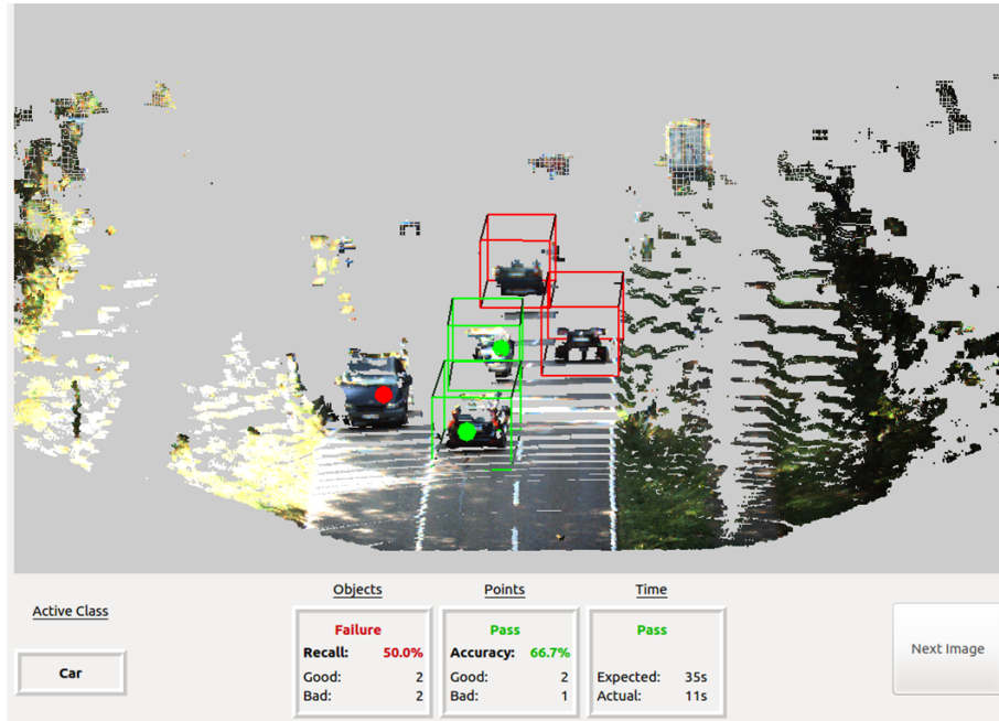
Figure 3.3: The annotator assessment window depicts the annotators correct and erroneous attempts. The green bounding boxes with the green points indicate a proper annotation attempt. The red bounding boxes are missed object instances. The red point is an erroneous attempt that is not near to any of the correct instances.
