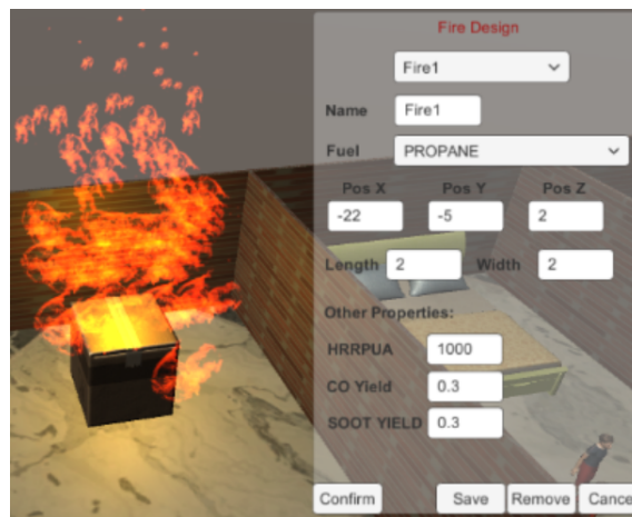
Figure 3.7: Fire design panel.
