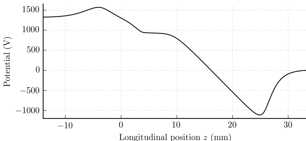
Figure 3.10: Simulated on-axis electric potential used to kick ions out of the analyzer trap.
