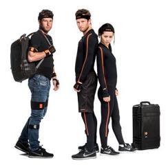
Figure 2.2. Photograph of the Xsens MVN Awinda (left) and Link (right) inertial MoCap systems
