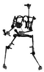
Figure 2.3. Photograph of Metamotion's Gypsy 7 exoskeleton MoCap system
