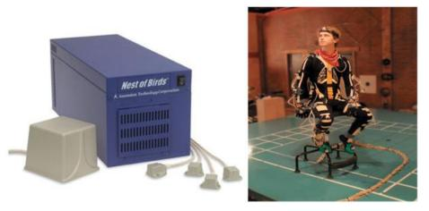
Figure 2.5. Photographs of the Nest of Birds magnetic MoCap system transmitter unit (left) and subject-interfaced sensor units (right)
