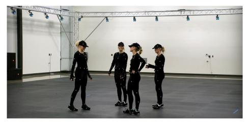
Figure 2.1. Photograph of an OptiTrack MoCap system with visible cameras below the truss structure and passive markers on the subjects
