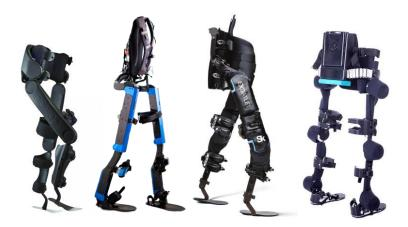
Figure 2.13. Photographs of the Indego (far left), Mina (middle-left), ExoAtlet (middle-right), and HANK (far right)
