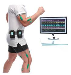
Figure 2.4. Photograph of Biometric's Ultimate Data Acquisition System based on wireless biaxial and monoaxial strain gauge sensors
