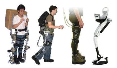
Figure 2.9. Photographs of the NTU-LEE (far left), MIT exoskeleton (middle-left), Donelan et al.'s exoskeleton (middle-right), and Bodyweight Support Assist (far right)
