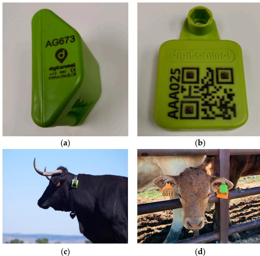
Figure 3. Hardware components of the solution: (a) GPS device detail; (b) BLE device detail; (c) GPS collar placed on the neck of a cow; and (d) BLE tag placed on the ear of a calf.
