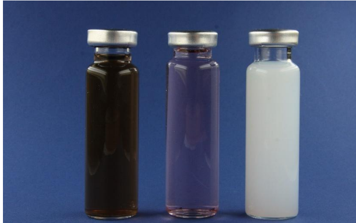
Fig. 1: Employed nanofluids. From left to right: GO, Au, and Al 2 O 3 -nanofluid.
