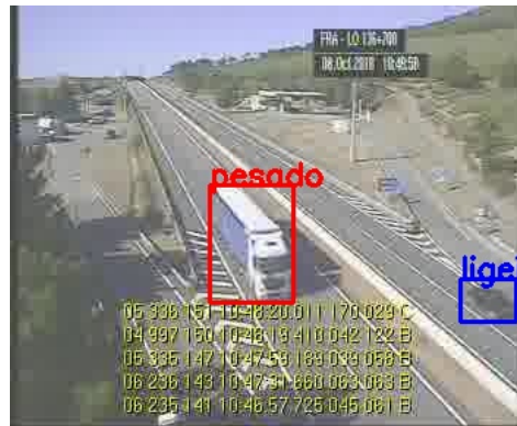
Figure 4.18: Example of prediction of SSD trained on all the datasets for dataset 1
