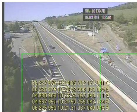
Figure 3.7: Regions chosen for background subtraction classification on dataset 1, area threshold is 1890 pixels
