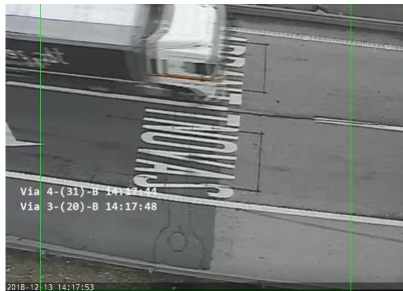
Figure 3.9: Regions chosen for background subtraction classification on dataset 3, area threshold is 60 000 pixels
